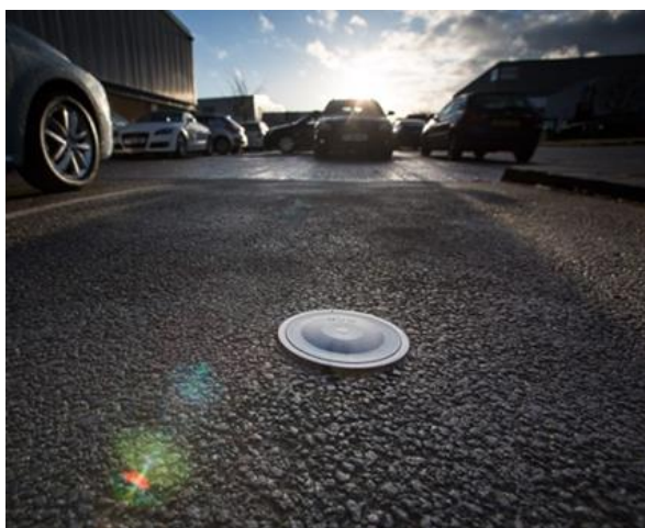
Figure 10.13 Example of a Parking Bay Sensor
